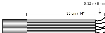
Figure 33: Insulation stripping – AC
