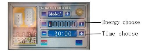
Technical Parameters Laser diode, wavelength: 635nm ~650nm Energy output :56 x 180mW Mains power output: 100VA Safety :On board diagnostics Classification :Electrical Class 1, Type B applied part Cooling requirements :Air cooled
