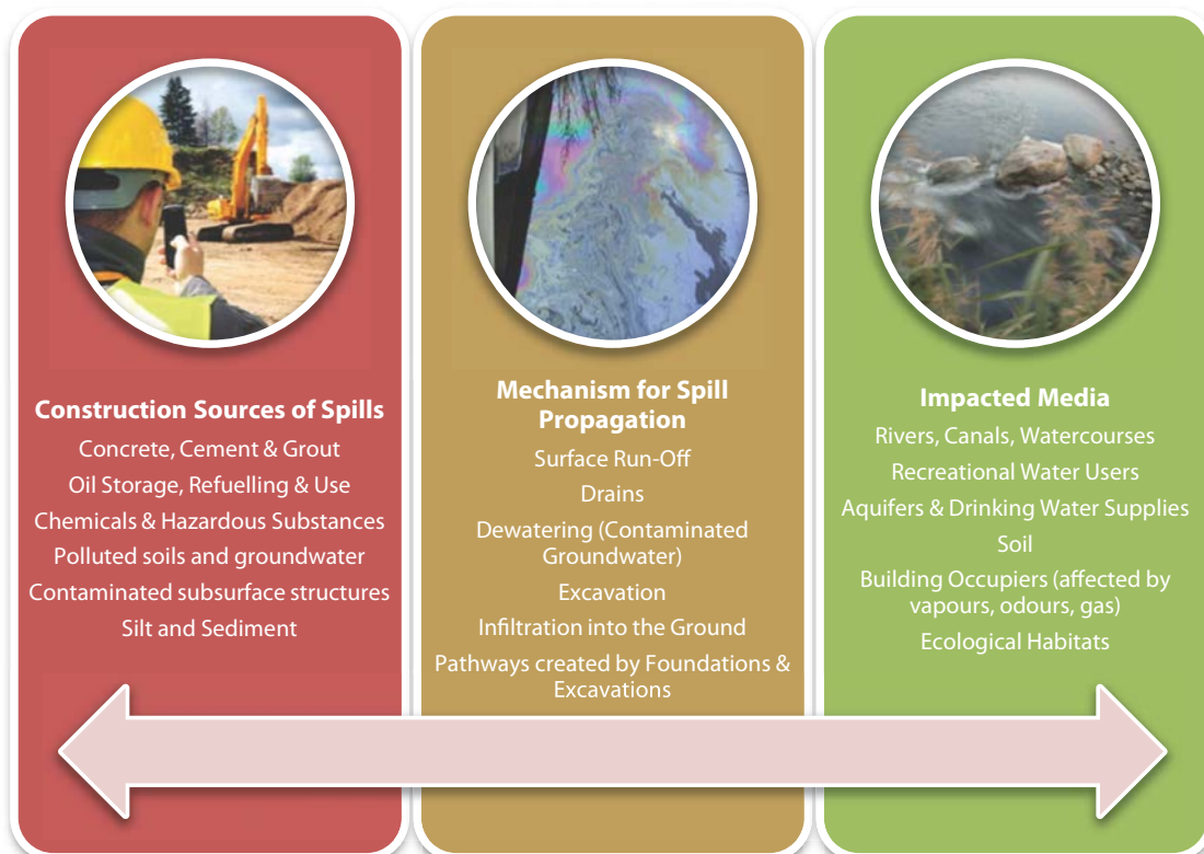
Figure 1: Sources, propagation and impacts of pollution spills
