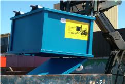
When working with large amounts of waste our auto dumping container range offers the greatest volume from the lowest overall size. Fitted with top mounted fork pockets and guides these units are easy to operate and the drop away base provides fast emptying.
