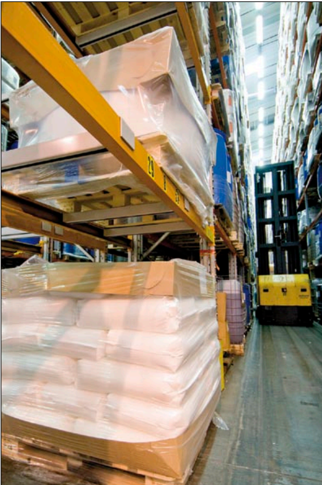
Figure 18 Narrow aisle fork-lift truck in operation
