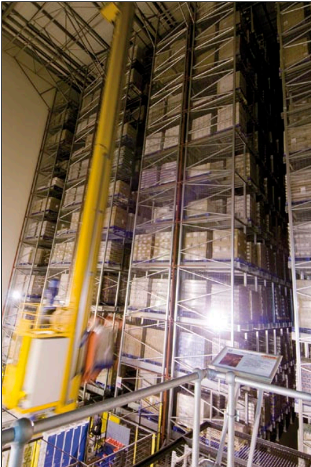
Figure 19 An automated narrow aisle fork-lift truck in operation
