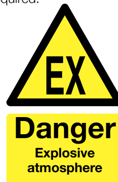
Figure 4 Example of warning sign with supplementary text used at entry points to locations where a potentially explosive atmosphere may exist
