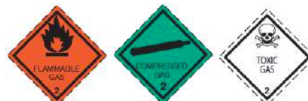
FLAMMABLE NON-FLAMMABLE/ NON-TOXIC TOXIC
