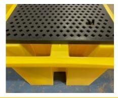
\*The grid should be placed up against and in-between the nodules at both ends of the pallet. There are 2 positioned at the front & 1 at the back (3 in total). These are designed to prevent the grid from moving or sliding, especially when an IBC is being loaded/unloaded.
