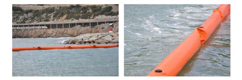
Typically deployed from response vessels where a foam filled boom would be too bulky, the reduced volume of an air filled boom is also an asset when they have to be transported as they take up comparatively little space. They are ideal for open water where the high buoyancy to weight ratio assists the performance in the waves and they have excellent UV resistance and chemical resistance to acids, alkalis, solvents and hydrocarbons.
