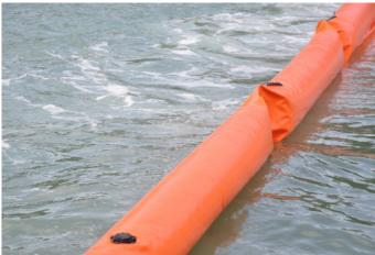
Typically deployed from response vessels where a foam filled boom would be too bulky, the reduced volume of an air filled boom is also an asset when they have to be transported as they take up comparatively little space. They are ideal for open water where the high buoyancy to weight ratio assists the performance in the waves and they have excellent UV resistance and chemical resistance to acids, alkalis, solvents and hydrocarbons.
