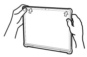
STEP 2: Press the device into the case skin as illustrated. Ensure all edges and features of the device and case skin are properly aligned. The device will snap completely into the case's perimeter seal.
