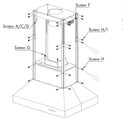
NOTE: Island range hoods with single motors will come with a square to 6" round transition piece and will include a back draft damper. The ducting with these range hoods is 6". Dual motor island hoods will come with a square to 8" round transition piece and in some instances are fitted with a built-in damper. For existing installations that may already have an external damper. Please consult an HVAC or installation professional for advice to comply with local regulations.
