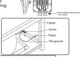
The bathtub must be connected to the ground. Power outlet must be sealed well.
