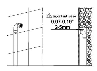
5.Install shower arm and rain shower head(wrap the PTFE tape on the thread
