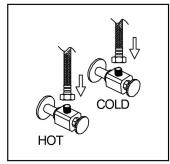
5. Attach flexible hose to water supply.
