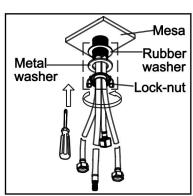
2. install the rubber washer followed by the metal washer and lock-nut. Hand tighten then tighten further using a screwdriver to tighten lock-nut screws.
