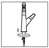
1. Take the product out of the packaging box, put the pull tube and water inlet pipe into the reserved hole for installation, and then put the faucet into it.
