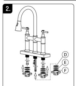
2. Use a nut (F) to fix the faucet. Rubber washer (D) and metal washer (E) are needed between the nut and fixed plate.
