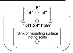
The faucet fits for Ø1.38" installation hole. The distance of this two installation hole is 4". Please see the below photograph as marked.
