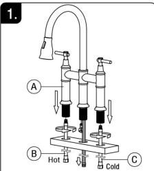
1. Connect the hot and cold supply hoses(B&C) to the main body (A). Then put the main body into the installation hole and prepare the next step.
