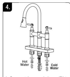
4. Connect the supply hose (B) to the hot water valve, connect the supply hose (C) to the cold water valve. Product installation is completed.
