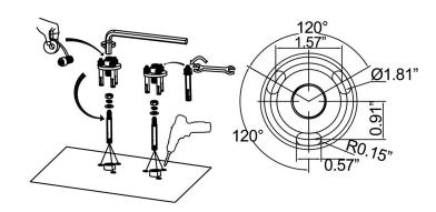
3. Screw the straight tube to the fixed assembly.
