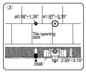
2. The maximum and minimum distances from the bottom of the concealed box to the decorated wall are shown in Pic 2.
