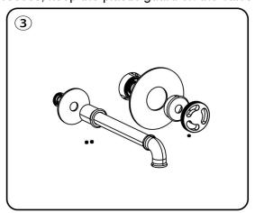
3. As shown in Pic 3, after finishing the wall decoration, install the decorative sheet, trim plate, spout and handle correctly.
