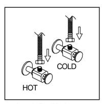
5. Attach flexible hose to water supply.
