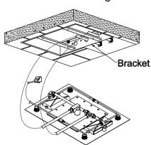
12. Lock the shower assembly onto the bracket with a hexagonal spoon. And the power plug in the plug board after power; Put in the drywall.
