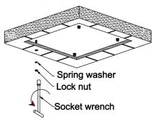
5. Move the bracket upward so that the four expansion screw heads pass through the four holes of the bracket.
