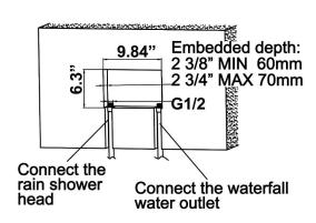
2. With reference of the basic size of the product, drill four Ø0.4" (10mm) holes in the appropriate position on the wall.
