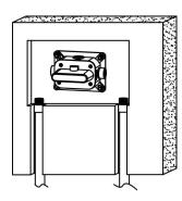
5. Rely on the spirit level to adjust the embedded main body on the horizontal line, use a sleeve to lock the 4 nuts to fix the embedded main body on the wall.
