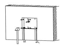
4. The pre-embedded body is supported by hand and installed on the four explosion bolts.
