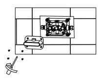
10. Insert the parts of shower head into the pre-embedded main body according to the corresponding hole.
