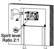
6. Put 1/2 flat spacer into the pre-embedded main body and tighten the water inlet joint.
