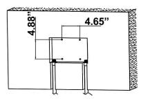
3. Drive four explosive bolts into the drilled holes with a hammer.
