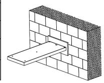
1. When customer receives the product, loosen the M6X8 screw with an Allen key as shown above.
