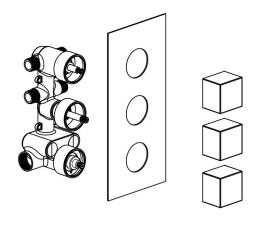
3. With reference to the basic dimensions of the embedded body, excavate the embedded ports of the main body, hot & cold water inlet pipe and the outlet pipe.
