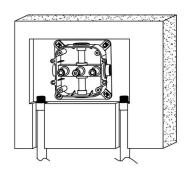
5. Attach the washers and spring gasket to the explosion screws, then lock the nuts into the embedded body with copper sleeve wrench.
