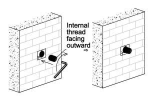
5. Install the remaining side sprinklers according to the previous steps.
