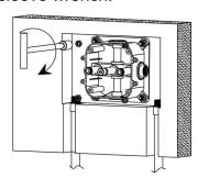
6. Put the 1/2 gasket into the pre-embedded body, and then tighten the water inlet pipe connector.
