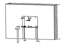
4. Put the embedded body into the position.
