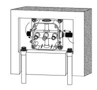
7. Connect waterlines properly then check leakage.
