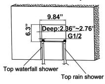
2. According to the size, Drill four (Ø10) holes on the wall.
