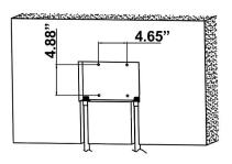
3. Hit the 4 explosion screws into the holes.
