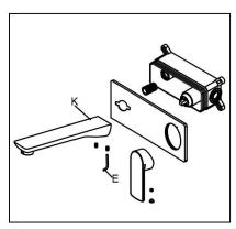
5. Fix the spout (K) to the position block and the thread pipe, and then use the Allen key (E) to tighten the spout with the thread pipe.
