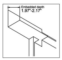
1. Holes size for the built in control valve: 6.89"x2.95"x(1.97"-2.17"), the depth between the bottom of the control valve to the tile surface is 1.97"-2.17".
