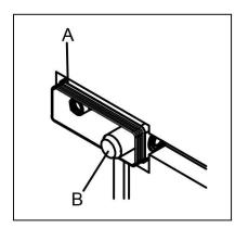
2. Use the tape on pipe threads, connected to the main body (A) cold and hot as required inlet pipe and outlet pipe, checking the leakage before fixing the main body in the embedded hole (keep the horizontal and vertical). And assembling the protection plastic cover (B).
