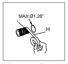
4. Wrap nylon tape (H) around the screw thread at the end of thread pipe, and then tighten the thread pipe (I) to the water pipe.
