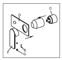
3. Remove the prastic cover (D) and then put the base through the cartridge cover (C), use Alleny key (E) and the hexagon socket screw to assemble the handle (F) to the body, and then put on the decorative button (G).
