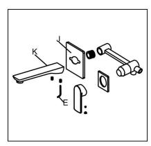
5. Remove the plastic cover (J) and then fix the spout (K) to the position block and the thread pipe, and then use the Allen key (E) to tighten the spout with the thread pipe.
