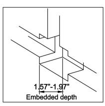
1. Holes size for the built in control valve:2.76"X2.36"X(1.57"~1.97"), the depth between the bottom of the control valve to the tile surface is 1.57~1.97".
