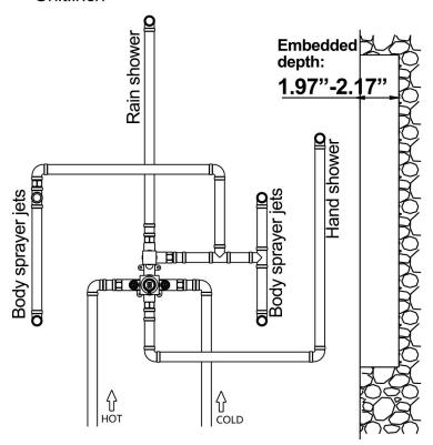
5. Install the upper outlet pipe and the top shower head.(wrap the PTFE tape on the thread)
