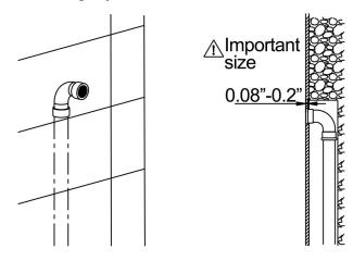
5. Determine the location of the mounting hole according to the actual size, and drill a hole in the wall.
