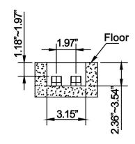
4. Connect the inlet tube like the drawing.
