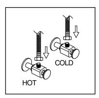
5. Attach flexible hose to water supply.
