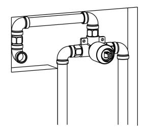
4. The water outlet of the waterfall is slightly lower than the tile surface.
