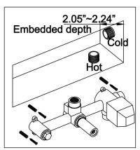
1. Open holes [size of opening is (10.43"-10.71")x(3.62"-3.78")x (2.05"-2.24")inch (LxWxD)] and embedded water pipes (hot and cold inlet pipes, outlet pipes) as required; Install the main body in the embedded hole and connect the pipe.
