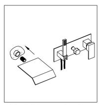
5. Install the spout to the outlet in the wall.
