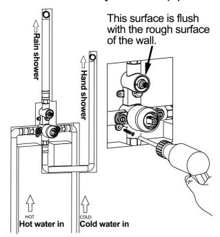
3. The water outlet is slightly lower than flat on the tile surface.
