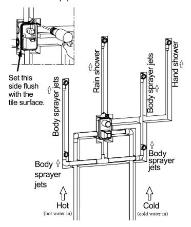
3. After fixing ceramic tiles, cut off edges of the embedded box, remove the protective cover and install the panel.
