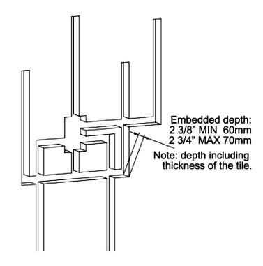
2. Install the main body, water inlet pipes and other pipes.
