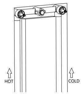
3. Fix the main body of the faucet with self-tapping screws (the main body must be flush with the wall).
