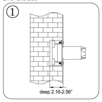
3. Connect the inlet and outlet pipes as shown in the picture
