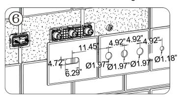
7. As shown in the picture, install flange, diverter handle and cartridge handle.
