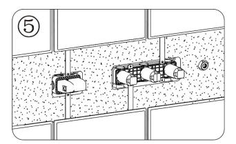
6. As shown in the picture, affix the tiles, and open three holes with a diameter of 5cm in the middle tile, with a distance of 12.5cm between the two holes.
