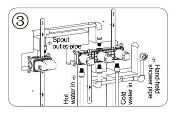
Before installing the faucet, please be sure to remove sundries and sludge from the water pipe to prevent sundries from blocking the faucet.
