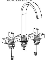
4. Connect the pipe of spout and two handles.
