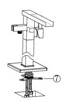
6.Drill holes on floor based on the drawing.
