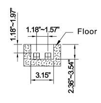
4. Connect the inlet tube like the drawing.
