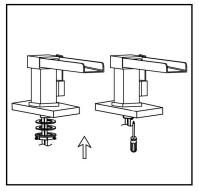
4. Re-install the rubber washer followed by the metal washer and lock-nut. Hand tighten then tighten further using a screw driver to tighten lock-nut screws.
