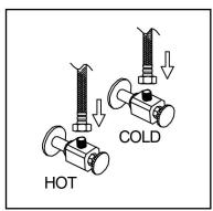
5. Attach flexible hose to water supply.
