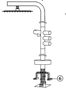
Drill holes on floor based on the drawing.
