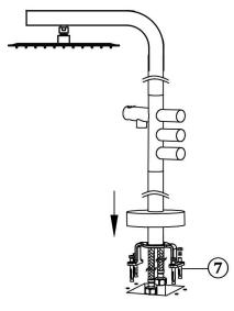
2. Screw the shower head into the connecting pipe, then connect the connecting pipe to the main body, and screw the main body to the straight pipe.
