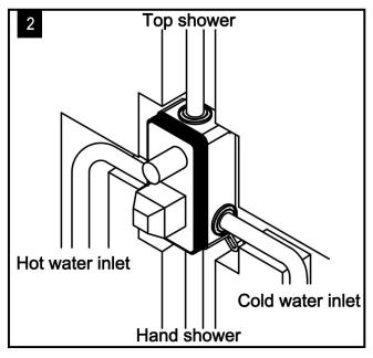
2 (1).According to the site condition and the installation size requirement to set up the pipe line. (2).Connect the embedded box to the pipe, put the embedded box on the hole, then adjusted the levels (the bubble on the middle of the leveller). (3).Make the positioning holes.
