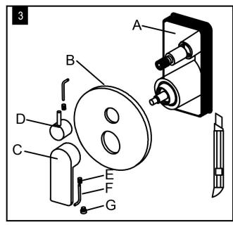
3. Remove the protective cover when the wall is completed and install the escutcheon (B) to the valve (A) and press it against the finished wall. Then, install the handle (C) and diverter knob (D), tighten set screws (E) with Allen key (F), and put on the indication buttons (G).
