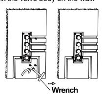
8). Connect all the pipes to check leakage, confirm no leak occurs when turn on water.
