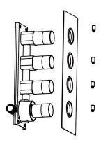
3). With reference to the basic dimensions of the embedded body, excavate the embedded ports of the main body, hot & cold water inlet pipe and the outlet pipe.
