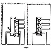
7). Use a Phillips screwdriver to tighten the 4 self-tapping screws, fix the valve body on the wall.
