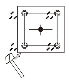
4). Fix the assembly to the ceiling wall with self-tapping screws .
