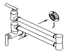
6. Connect the faucet to the thread joint on the wall, and use a hex wrench to tighten the screw from the side of the base to fix the base.
