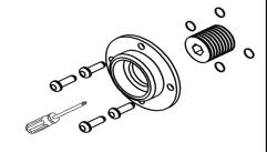
4. Fixing the base with screws
