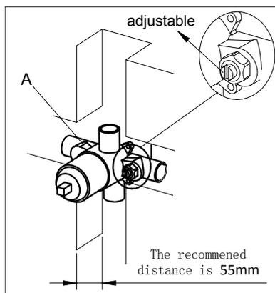
1. According to the site condition and the installation size requirement and to make a hole, the hole size is 100mm(length)\*130mm(width)\*55-60mm(deep).
