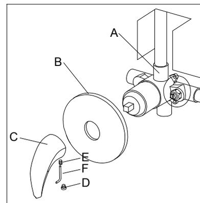
3. Remove the protective cover when the finished wall is completed and install the escutcheon (B) to the valve (A) and press it against the finished wall. Then, install the handle (C) tighten set screws (E) with Allen key (F), and put on the indication buttons (D).
