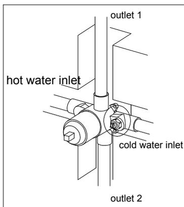
2. Wrap Teflon tape around the pipe threads and connect hot and cold water supply lines and in-wall pipes (not included) as desired to the valve. Turn on the water supply and open the cartridge to check for leakage. Then, put on the protective cover.
