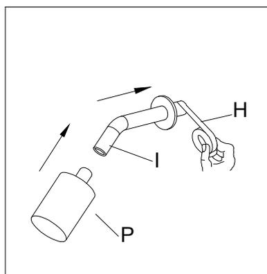
4. Turn the water on for 1 minute to flush any debris. Apply Teflon tape (H) to the threaded tail pipe and install the shower hose (I) into the outlet on the wall. Then connect the top shower (P) to the spout.
