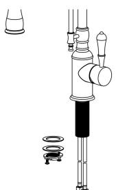
2. Pass the supply hose through the install hole.
