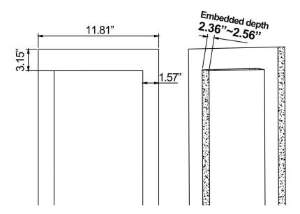
2. Install the main body and water inlet pipes.
