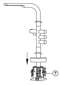
2. Screw the shower head into the connecting pipe, then connect the connecting pipe to the main body, and screw the main body to the straight pipe.
