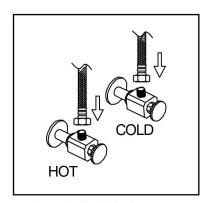
5. Attach flexible hose to water supply.
