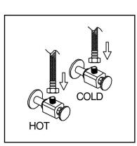
5. Attach flexible hose to water supply.
