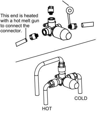
3. Put the valve body connected with the pipe against the wall, draw the outline with a pen and prepare for the slotting.
