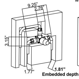
5. Drive the rubber plug into the wall, and fix the main body to the wall with screws.
