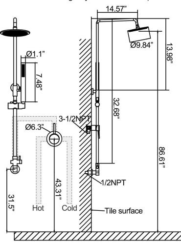
2. The connection between the valve body and the pipe needs to use the joint for the transfer function, and the joint needs to be sealed with a PTFE tape.
